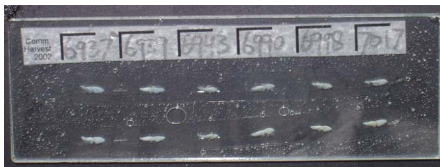
Figure 3.3 Two resin strips (System Three Clear Coat epoxy) each containing six sections of lake whitefish otoliths and a paper tag with the corresponding individual codes fixed between two microscopy slides (3" x 1") with System Three Clear Coat epoxy resin.
